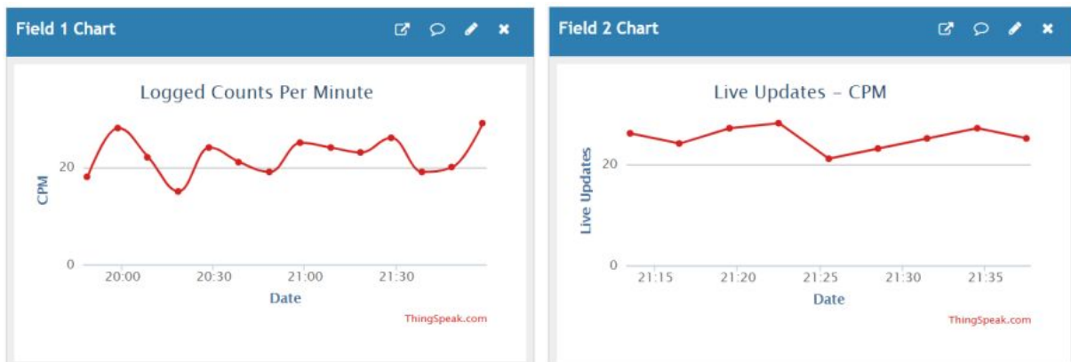
Figure 9: Examples of ThingSpeak data plots for logged data (left) and live upload (right)
